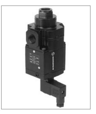
Materials: Body: Aluminium Intermediate body: Aluminium Elastomers: Synthetic materials Filter discs: Sintered plastic Internal components: Brass/steel Top plate: Zinc Exhaust bonnet: Zinc
